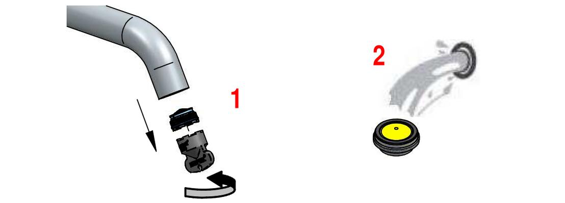
**! SOSTITUZIONE CARTUCCE / CARTRIDGES REPLACEMENT**
